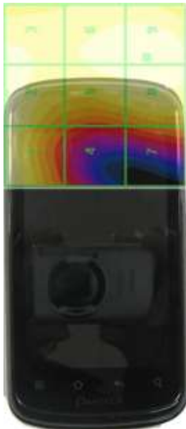
E-Field WD Scan overlay
