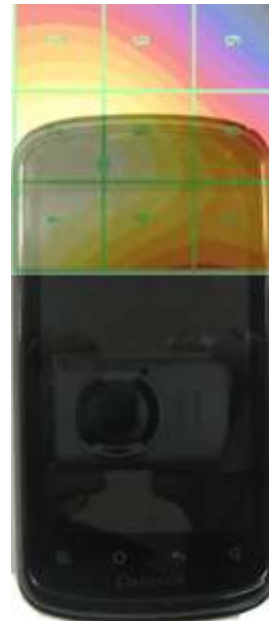
H-Field WD Scan overlay
