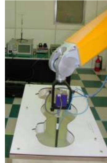
Figure 3.2 Photograph of the probe and the Phantom
