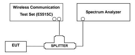
(Configuration of conducted Emission measurement)
