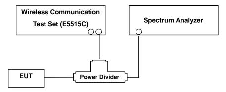
(Configuration of conducted Emission measurement) Test Procedure
