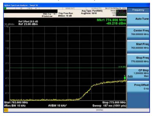
■ Upper Emission Mask (793 MHz - 805 MHz) 16-QAM -RB Size 50
