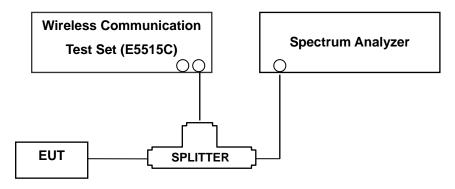
(Configuration of conducted Emission measurement)
