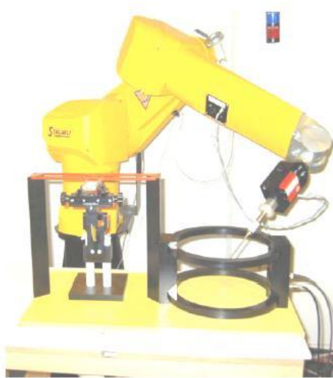
Figure 1: T-Coil setup with HAC Test Arch and AMCC.
