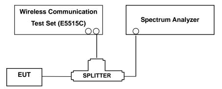
(Configuration of conducted Emission measurement)
