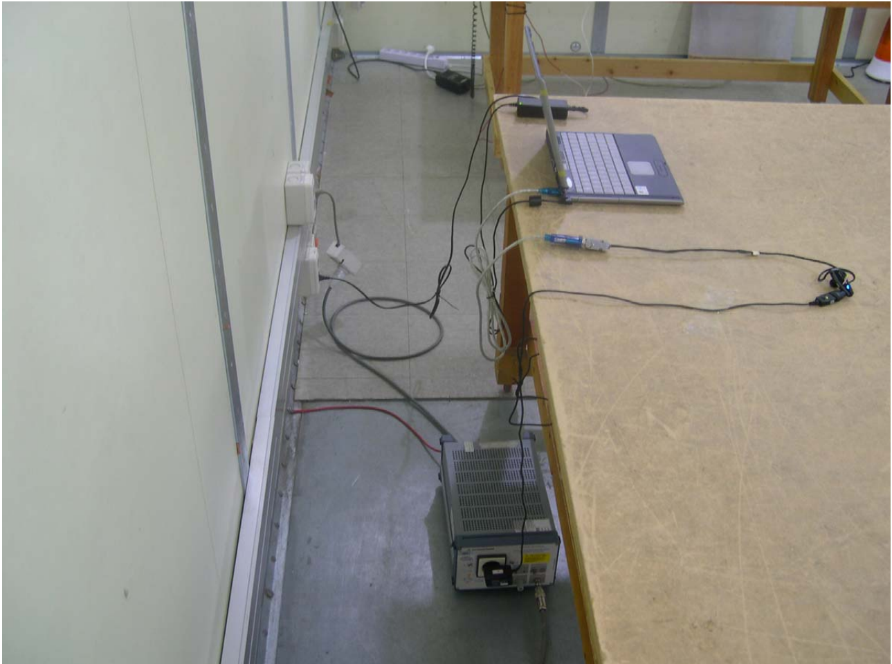
AC power line conducted emission measurement for AC/DC Adaptor #1; Model 5265C2-US Manufacturer: MCS ELECTRONICS CO LTD
