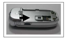
3. If you want to remove the SIM card, push the SIM card in the arrow direction as shown in the picture below.
