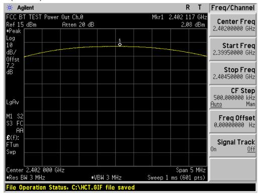
Test Plots (π/4DQPSK) Peak Power (Mid-CH)
