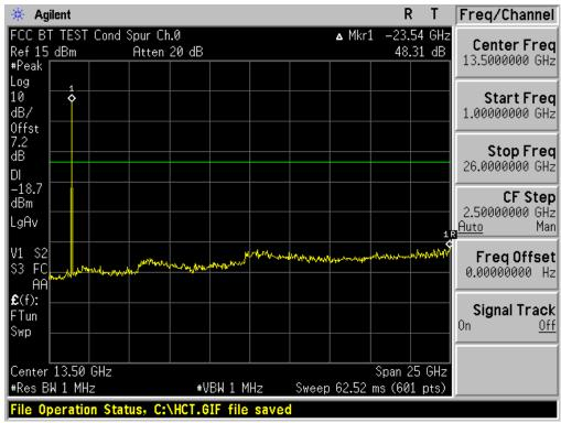
Test Plots ( $\pi$ /4DQPSK) - 1 GHz - 26 GHz (RBW:1 MHz, VBW: 1 MHz) Spurious Emission (Mid-CH)
