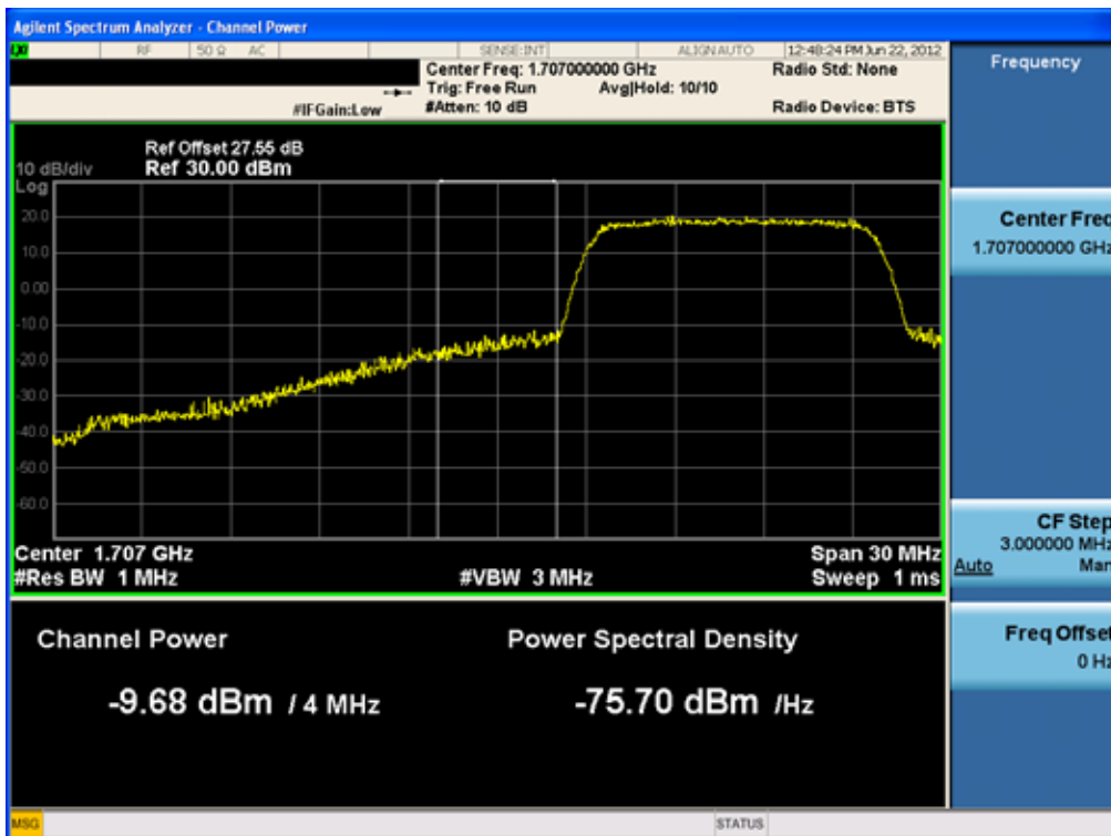
Lower Extended Band Edge Plot (10MHz QPSK – RB Size 50, Offset 0)
