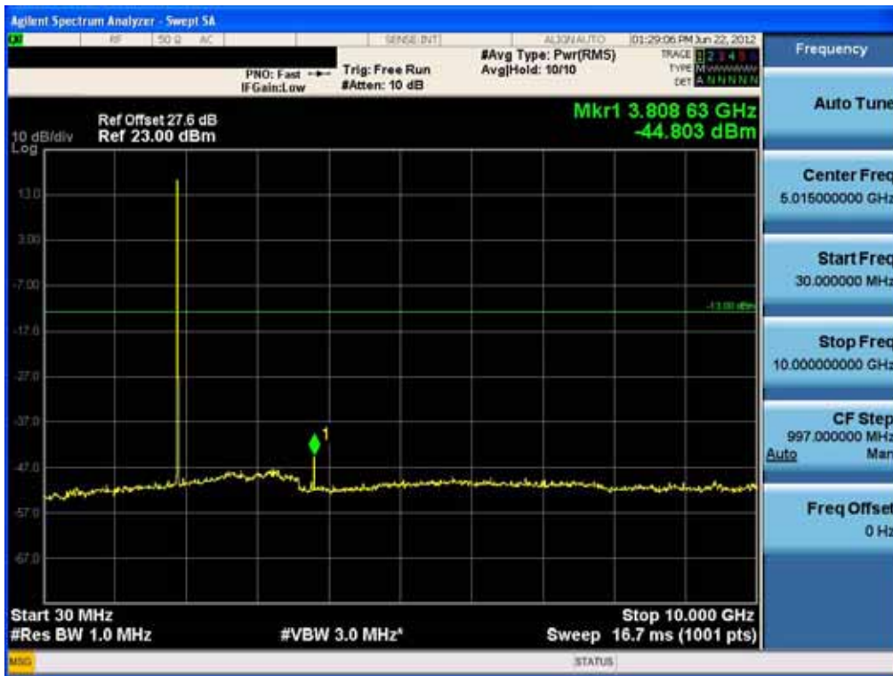
Conducted Spurious Plot (5MHz QPSK - RB Size 1, RB Offset 0 - High Channel)-1
