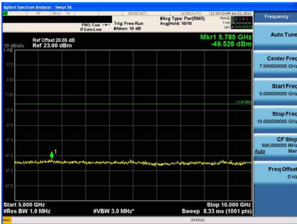
Conducted Spurious Plot (10MHz QPSK – RB Size 1, RB Offset 0 – Low Channel)-2
