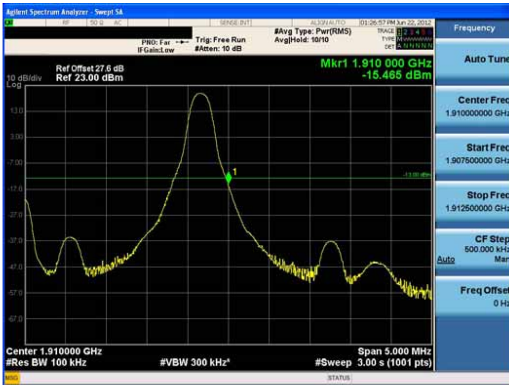
Upper Band Edge Plot (5MHz QPSK – RB Size 1, Offset 24)
