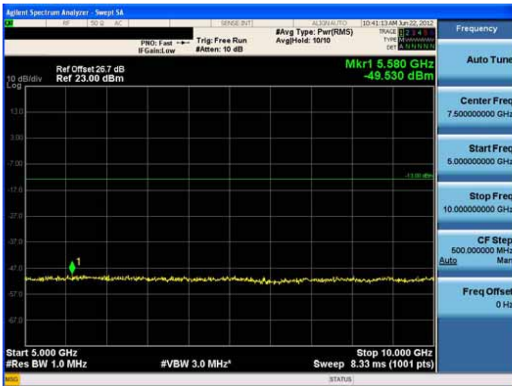
Conducted Spurious Plot (5MHz QPSK - RB Size 1, RB Offset 0 - Low Channel)-2
