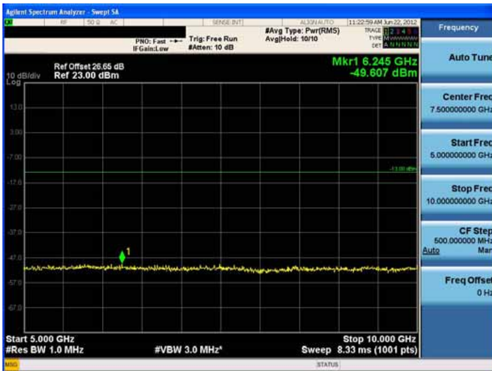
Conducted Spurious Plot (5MHz QPSK – RB Size 1, RB Offset 0 – Mid Channel)-2
