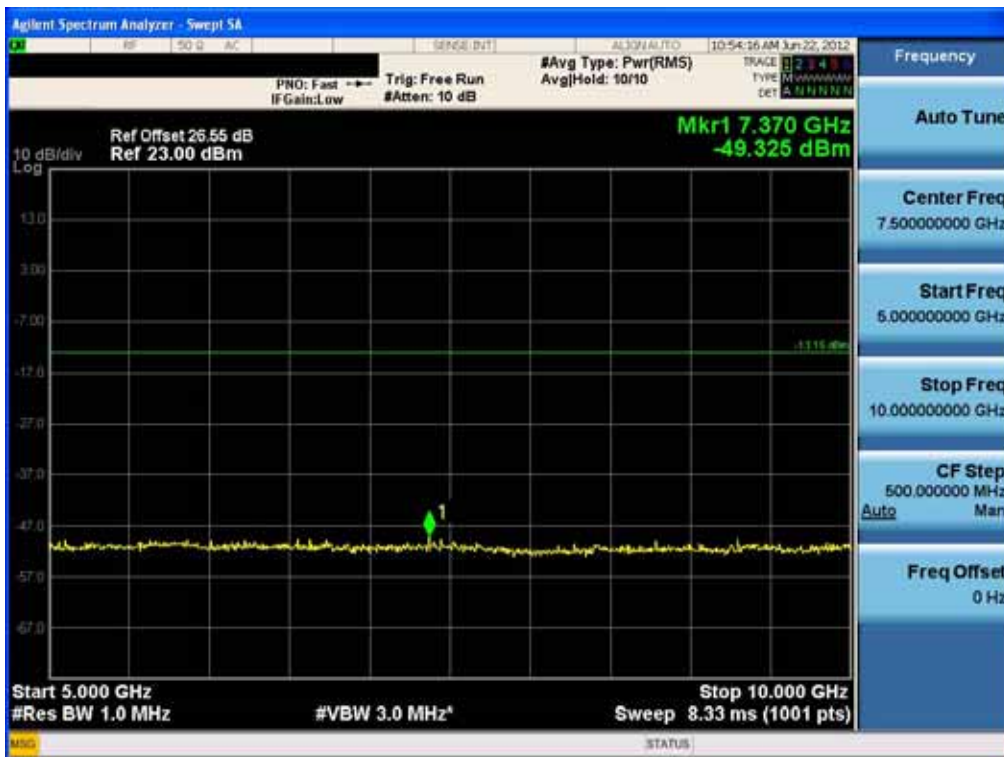
Conducted Spurious Plot (10MHz QPSK – RB Size 1, RB Offset 49 – Mid Channel)-2
