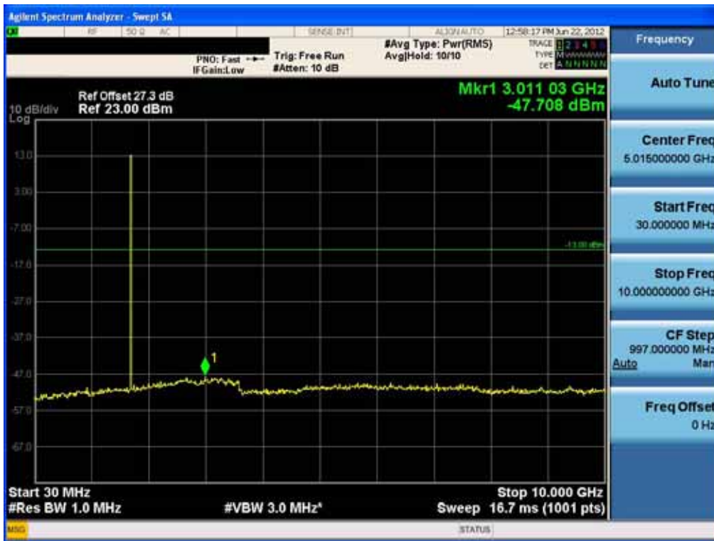
Conducted Spurious Plot (5MHz QPSK - RB Size 1, RB Offset 0 - Low Channel)-1
