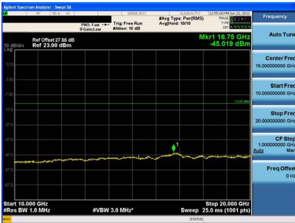
Conducted Spurious Plot (10MHz QPSK – RB Size 1, RB Offset 49 – High Channel)-2
