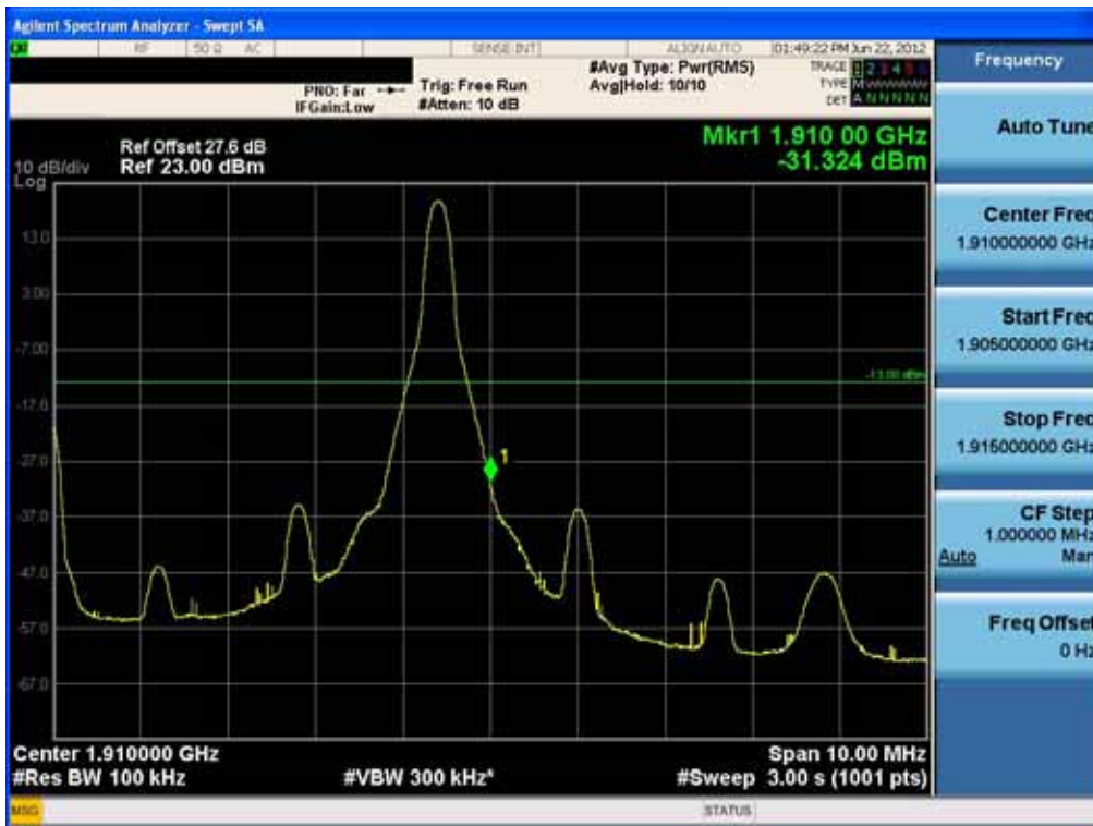
Upper Band Edge Plot (10MHz QPSK – RB Size 1, Offset 49)
