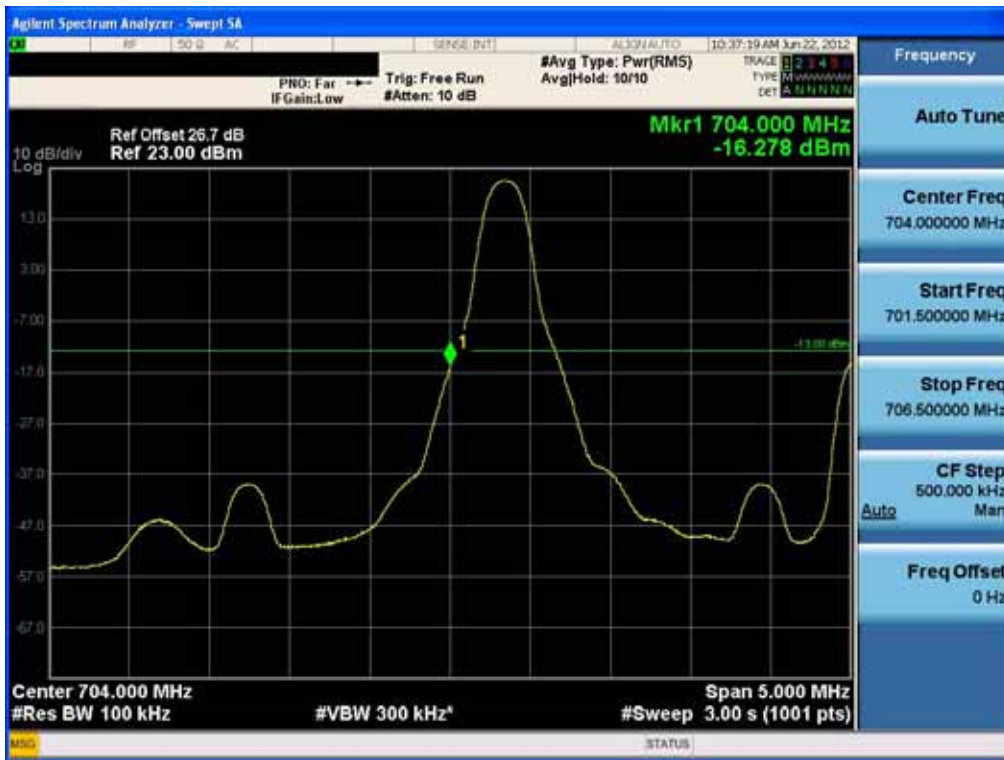
Lower Band Edge Plot (5MHz QPSK – RB Size 1, Offset 0)
