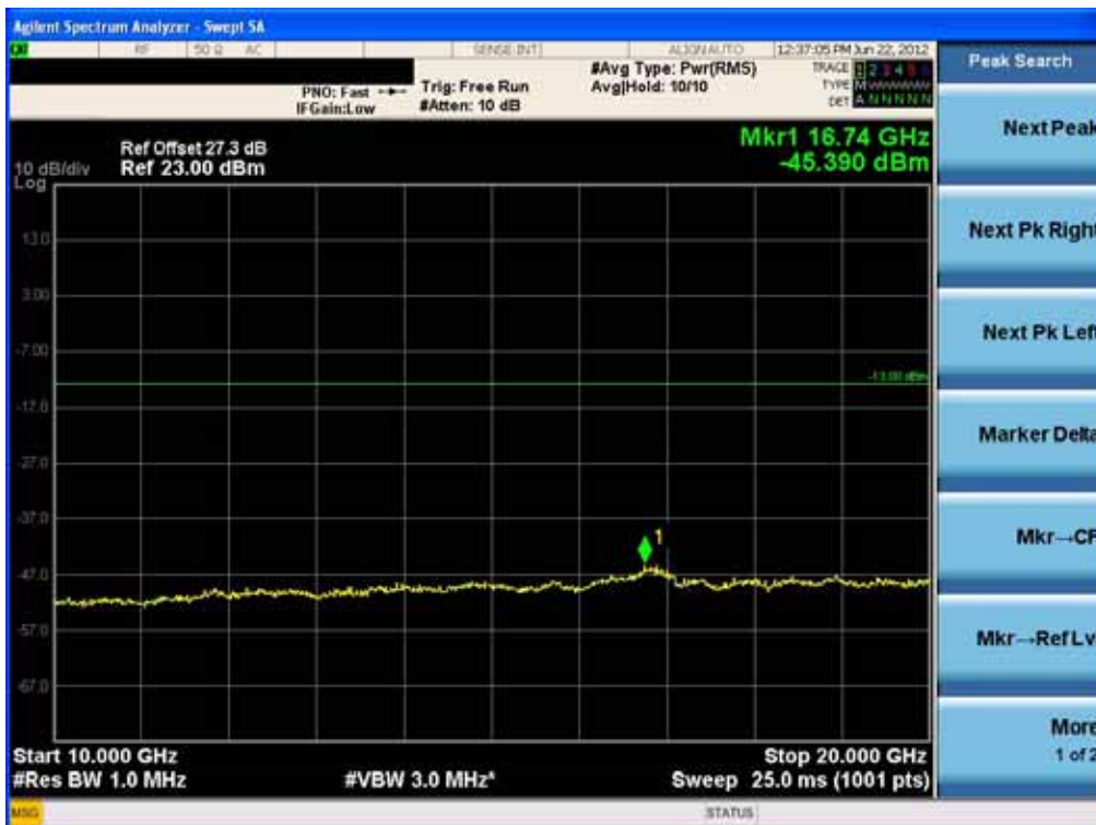
Conducted Spurious Plot (5MHz QPSK – RB Size 1, RB Offset 24 – Mid Channel)–2
