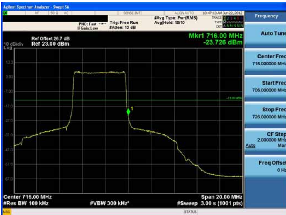
Upper Band Edge Plot (5MHz QPSK – RB Size 25, Offset 0)
