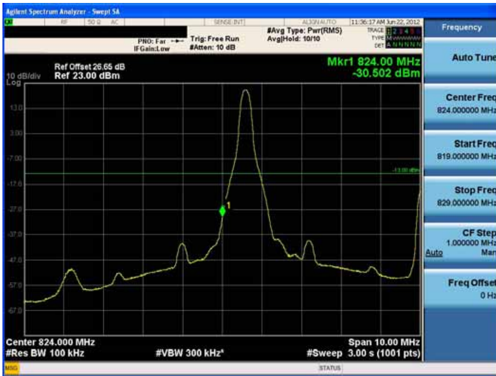
Lower Band Edge Plot (10MHz QPSK – RB Size 1, Offset 0)
