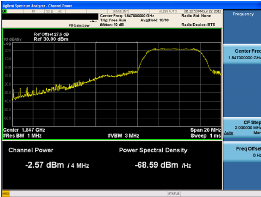
Lower Extended Band Edge Plot (5MHz QPSK – RB Size 25, Offset 0)
