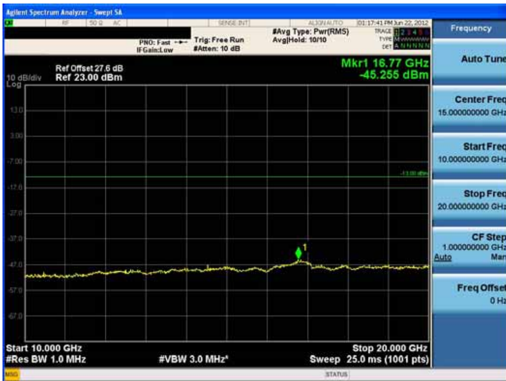
Conducted Spurious Plot (5MHz QPSK – RB Size 1, RB Offset 24 – Low Channel)-2
