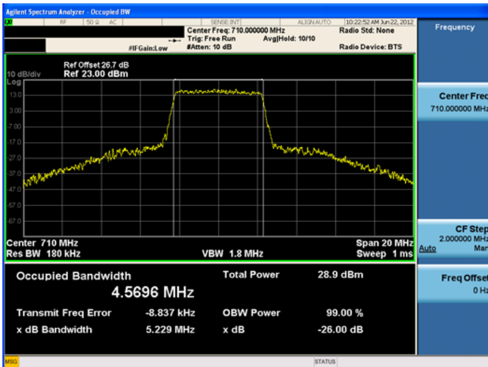
Occupied Bandwidth Plot (5MHz 16-QAM – RB Size 25)
