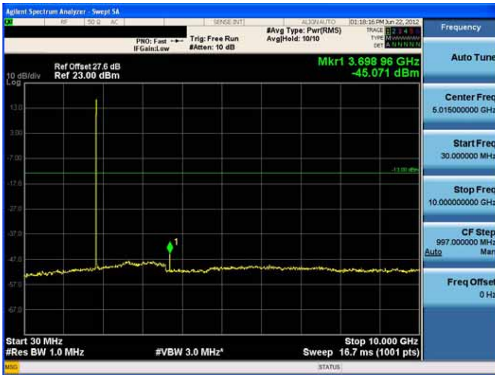
Conducted Spurious Plot (5MHz QPSK – RB Size 1, RB Offset 24 – Low Channel)-1
