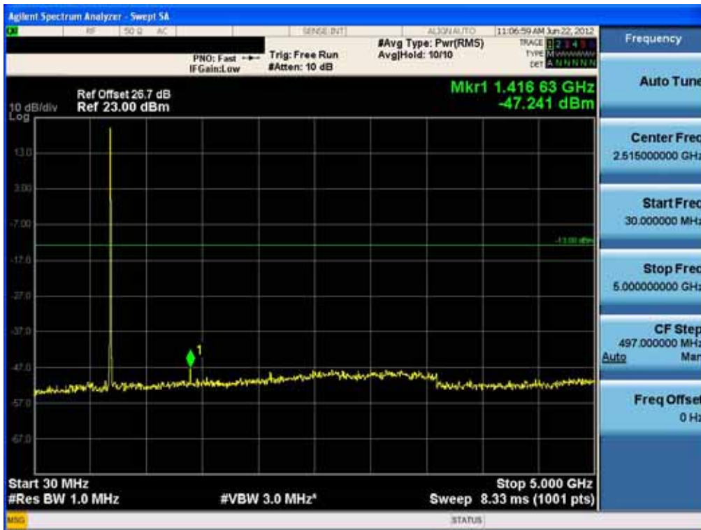
Conducted Spurious Plot (5MHz QPSK – RB Size 1, RB Offset 24 – Mid Channel)-1
