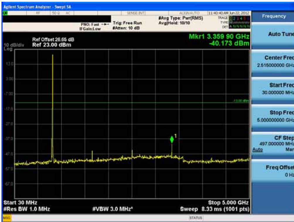
Conducted Spurious Plot (10MHz QPSK – RB Size 1, RB Offset 0 – High Channel)-1
