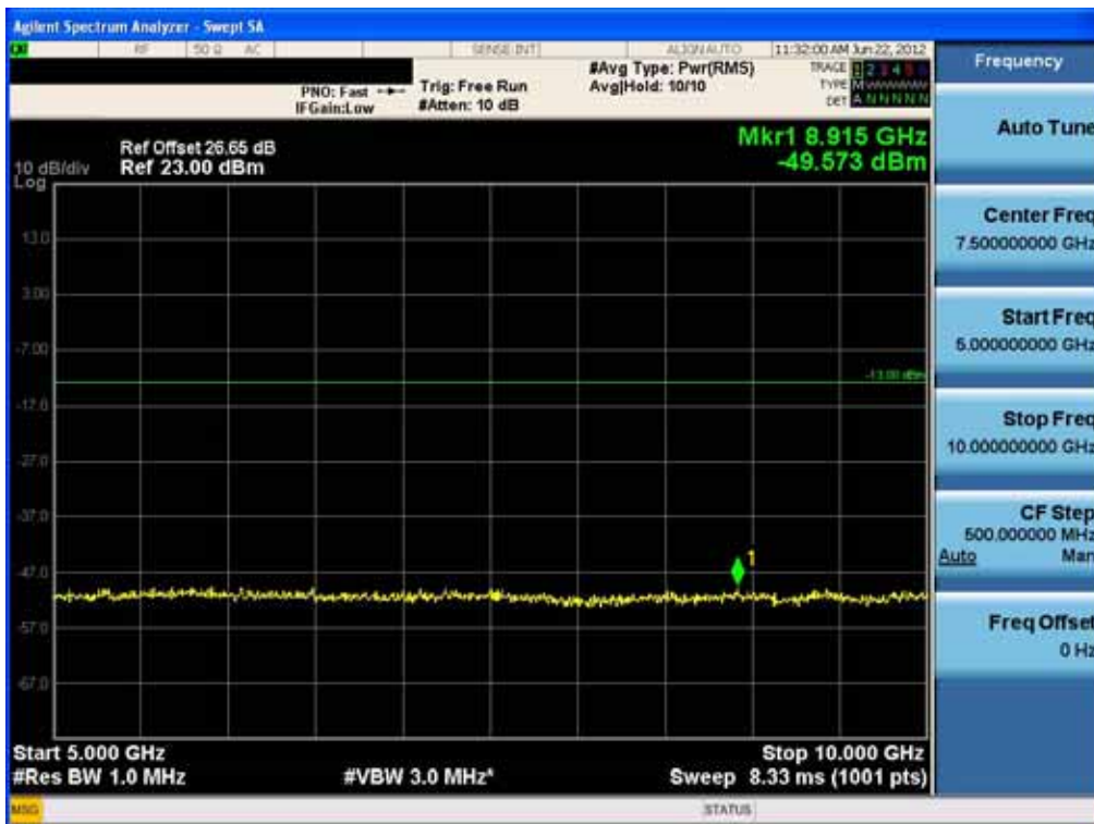
Conducted Spurious Plot (5MHz QPSK - RB Size 1, RB Offset 0 - High Channel)-2
