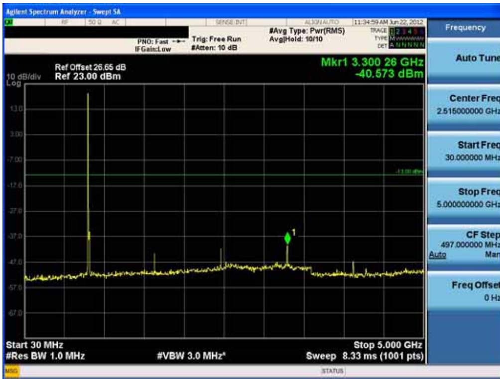
Conducted Spurious Plot (10MHz QPSK – RB Size 1, RB Offset 0 – Low Channel)-1
