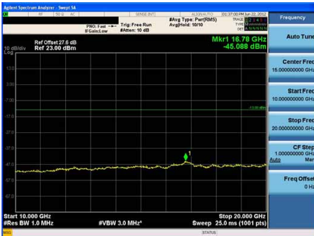
Conducted Spurious Plot (10MHz QPSK – RB Size 1, RB Offset 0 – Mid Channel)-2
