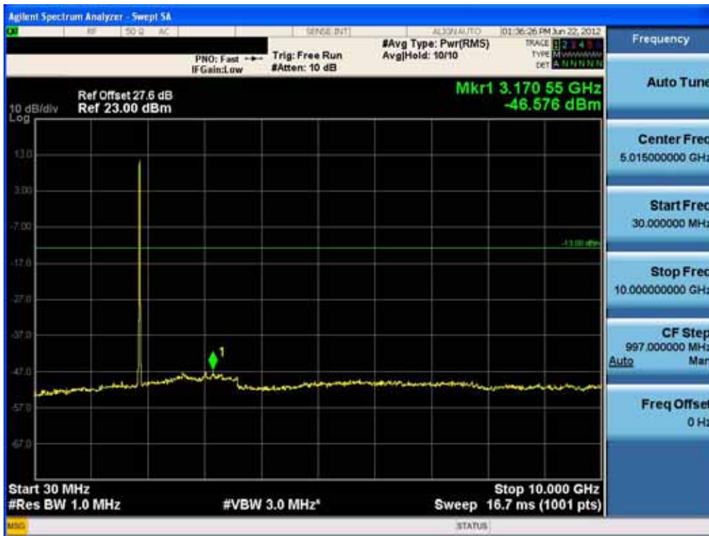
Conducted Spurious Plot (10MHz QPSK – RB Size 1, RB Offset 0 – Mid Channel)-1
