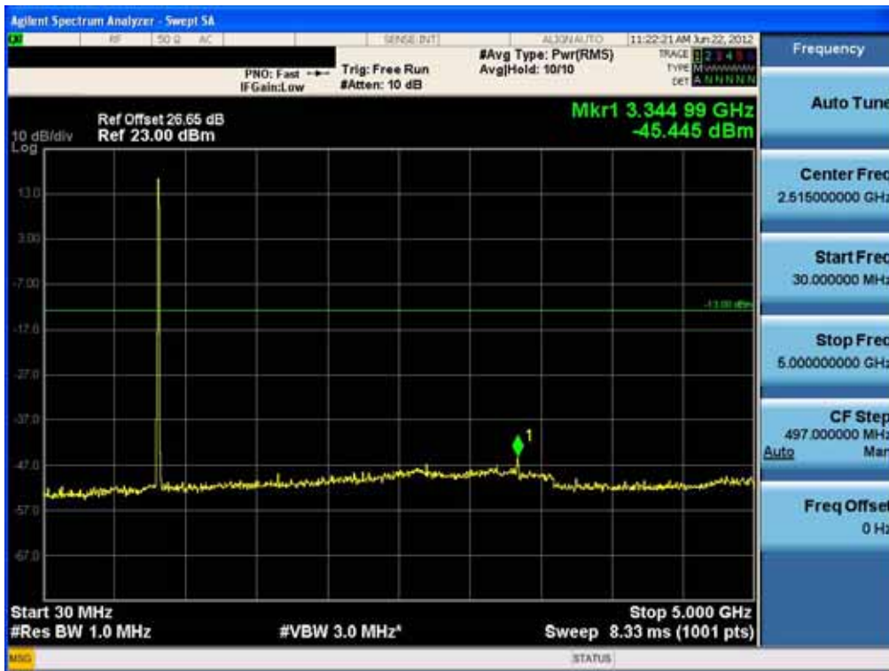
Conducted Spurious Plot (5MHz QPSK – RB Size 1, RB Offset 0 – Mid Channel)-1
