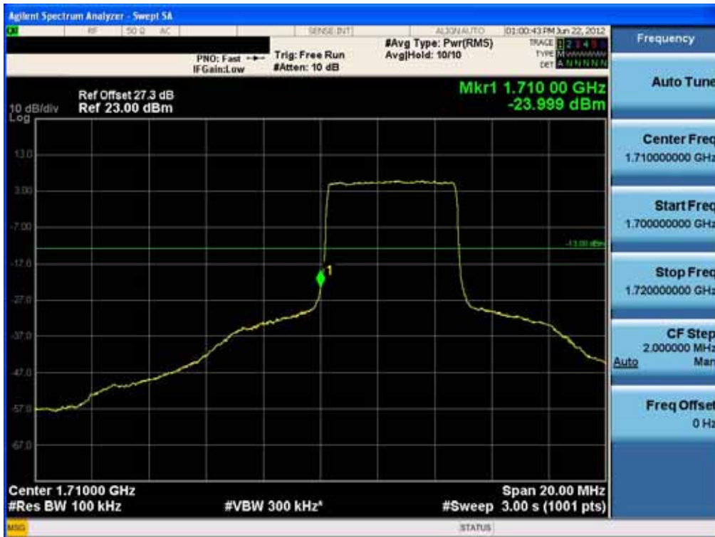
Lower Band Edge Plot (5MHz QPSK – RB Size 25, Offset 0)
