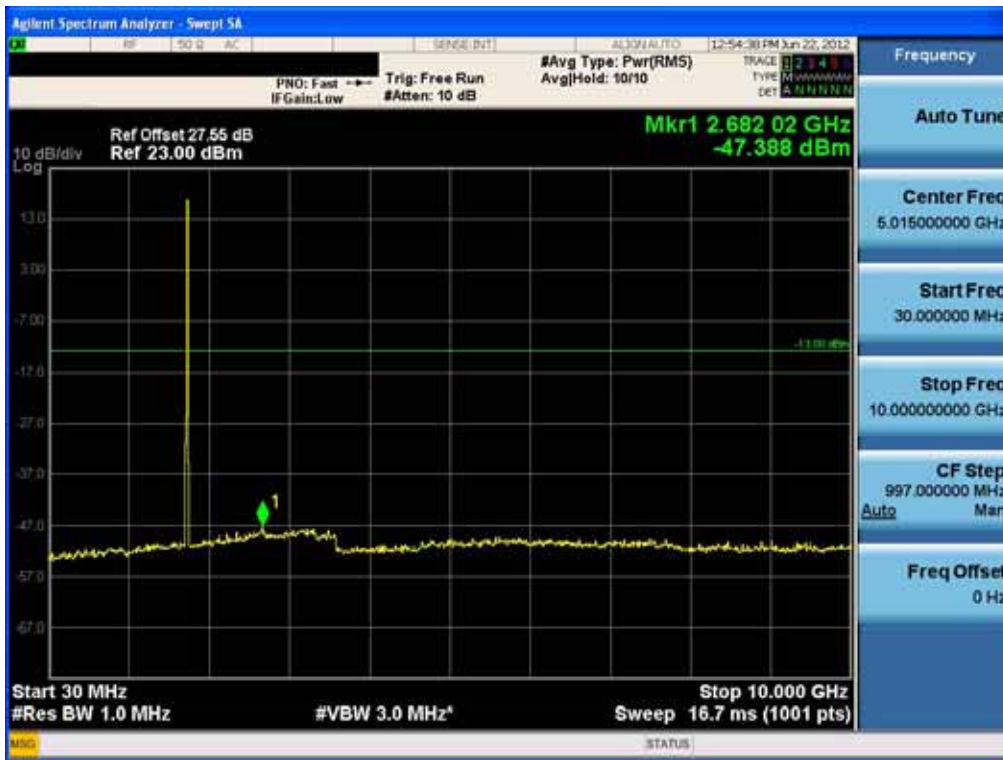
Conducted Spurious Plot (10MHz QPSK – RB Size 1, RB Offset 49 – High Channel)-1
