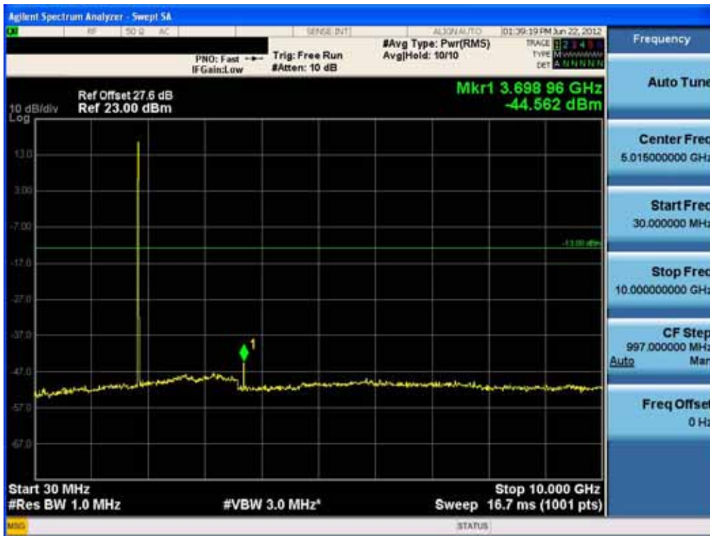
Conducted Spurious Plot (10MHz QPSK - RB Size 1, RB Offset 49 - Low Channel)-1
