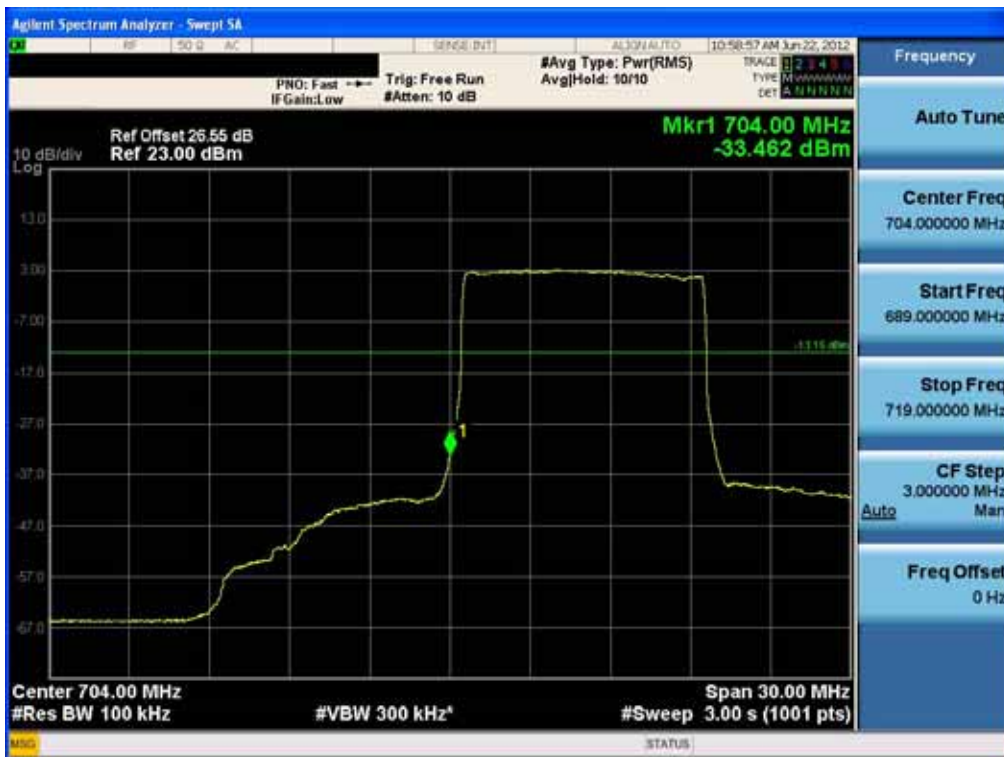
Lower Band Edge Plot (10MHz QPSK – RB Size 50, Offset 0)
