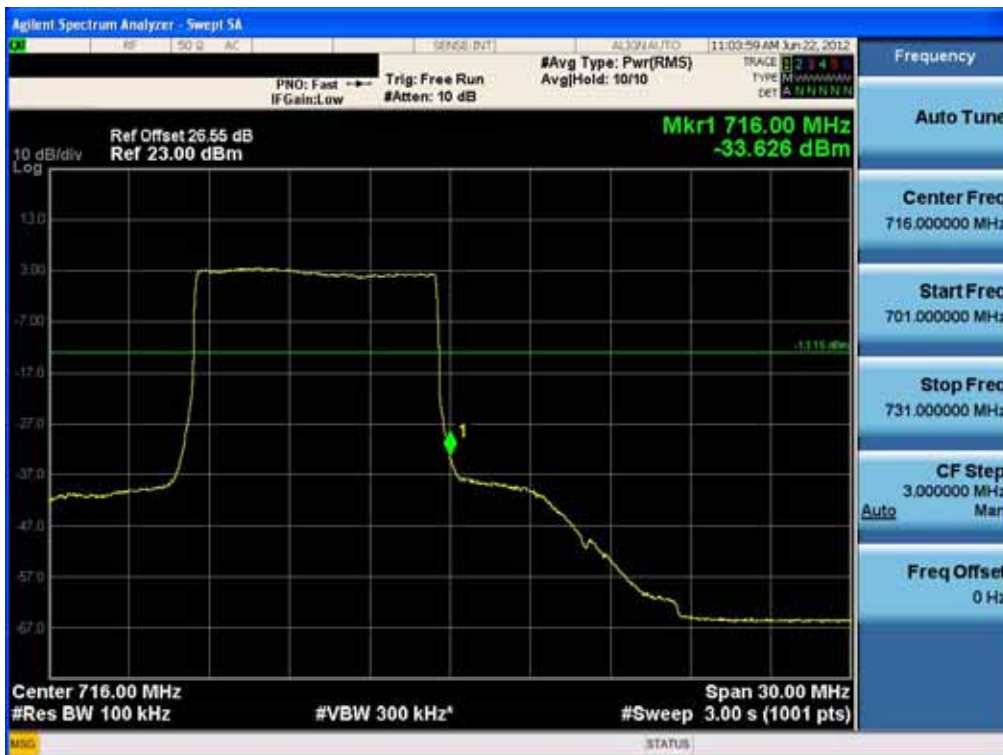
Upper Band Edge Plot (10MHz QPSK – RB Size 50, Offset 0)
