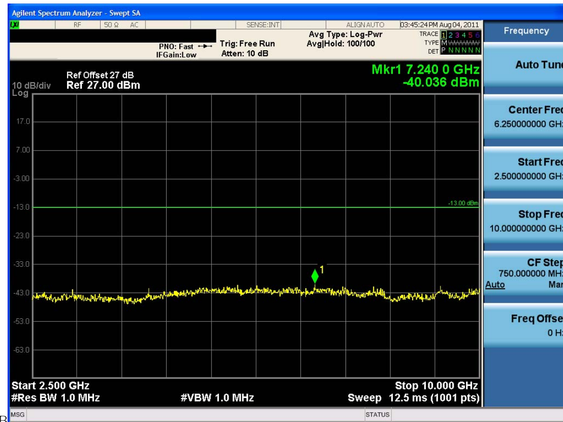
Conducted Spurious Plot (5MHz BW, QPSK, Band 5 – High Channel)
