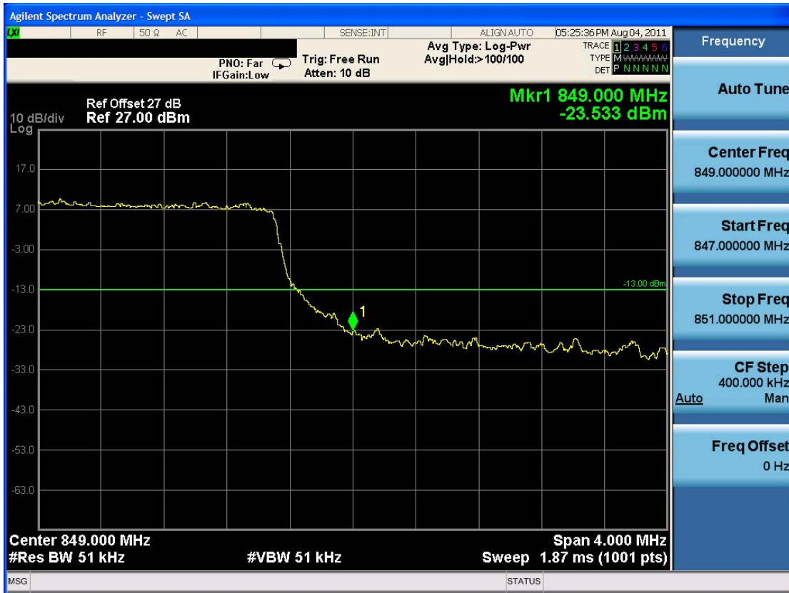
Band Edge Plot (10 MHz BW, QPSK, Band 5 – High Channel)
