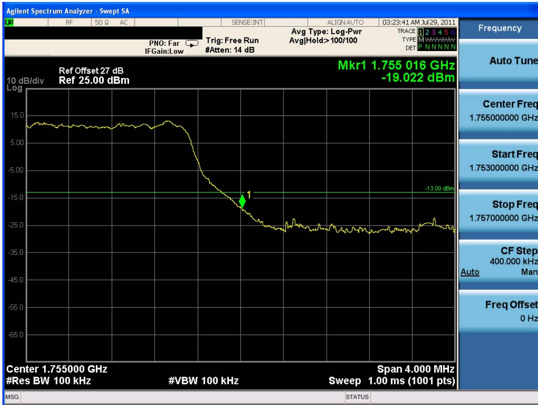
Band Edge Plot (10 MHz BW, QPSK, AWS Band – High Channel)
