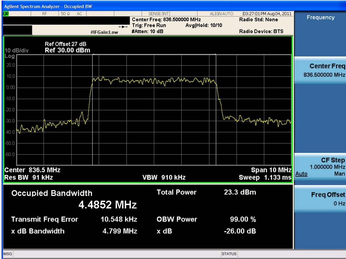
Occupied Bandwidth Plot (5 MHz BW, QPSK, Band 5 –Mid Channel)
