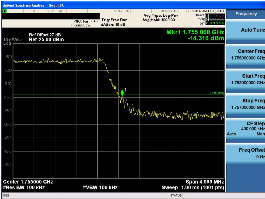
Band Edge Plot (5 MHz BW, QPSK, AWS Band – High Channel)
