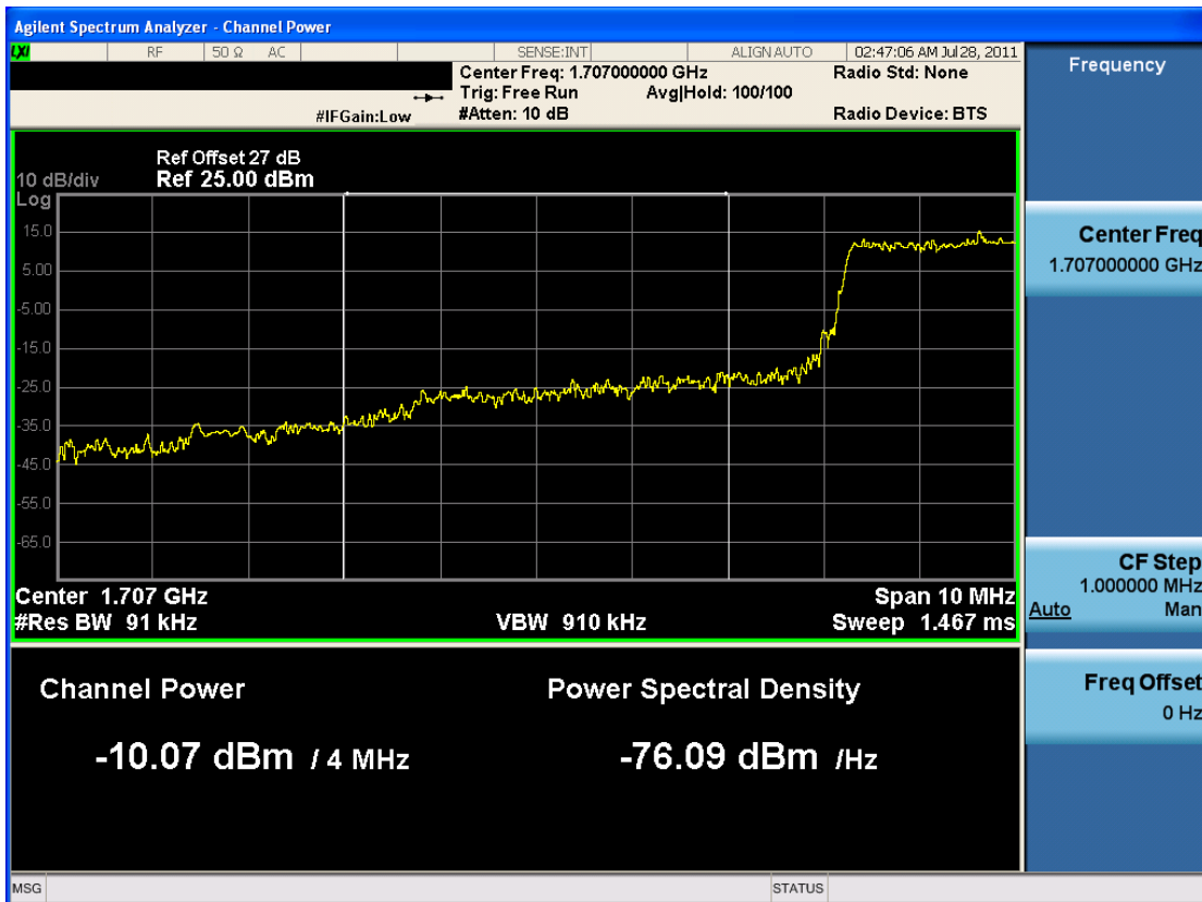
Extended Band Edge Plot (5 MHz BW, QPSK, AWS Band – Low Channel)
