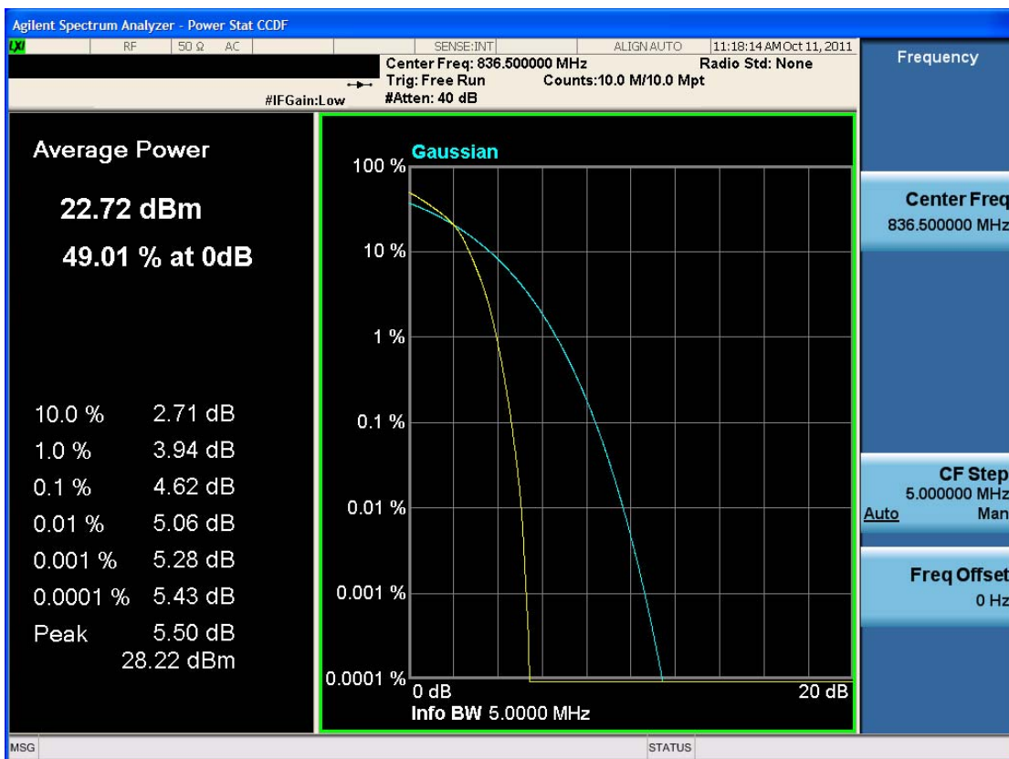
Peak-Average Ratio Plot (10 MHz BW, QPSK, Band 5 – Mid Channel)
