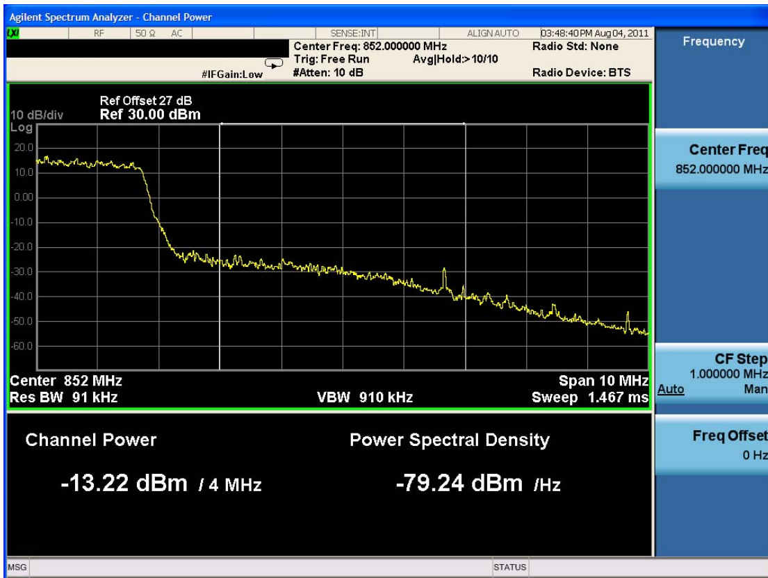
Extended Band Edge Plot (5 MHz BW, QPSK, Band 5 – High Channel)
