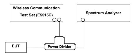
(Configuration of conducted Emission measurement) Test Procedure
