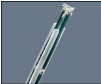
Figure 3.2 ES3DV3 E-field Probe
