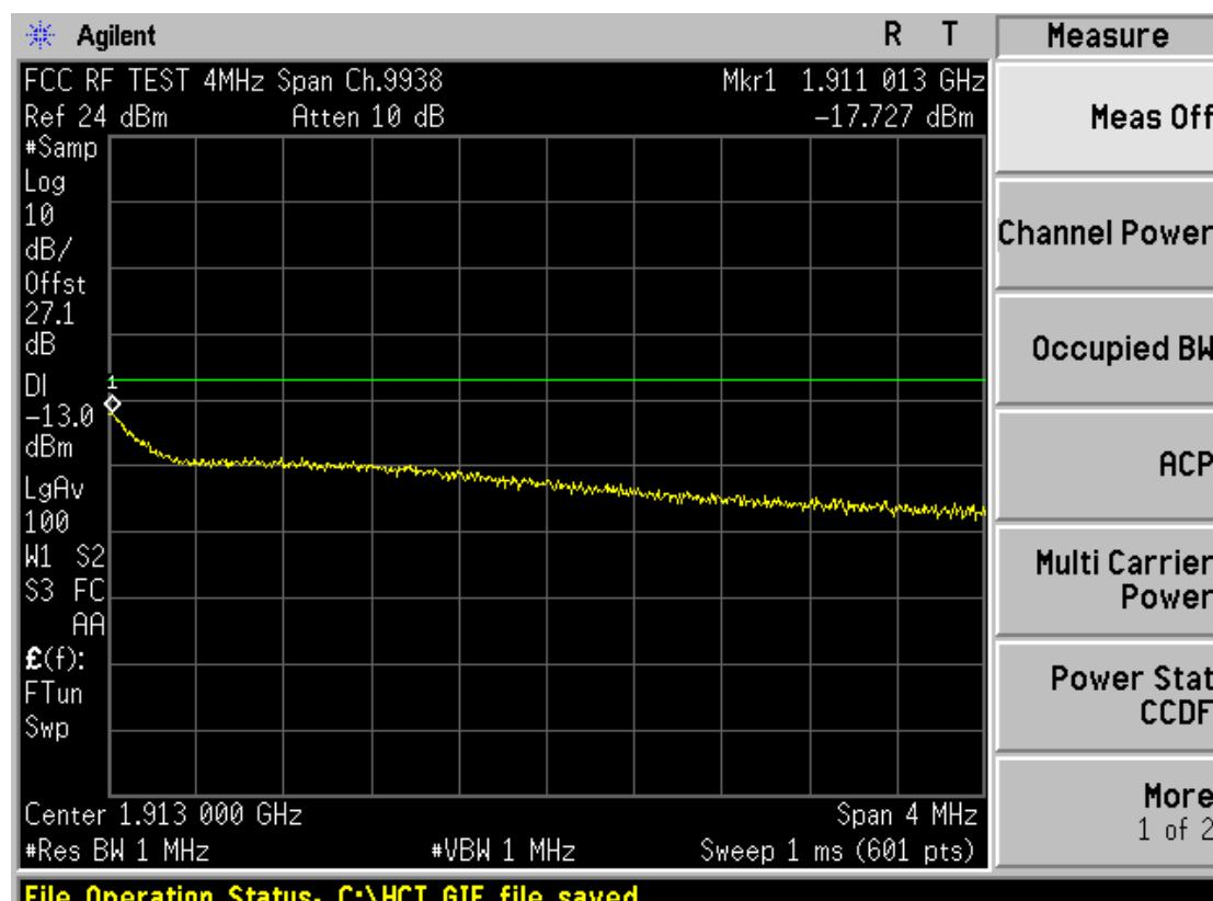
GSM850 MODE (128 CH.) Conducted Spurious Emissions1
