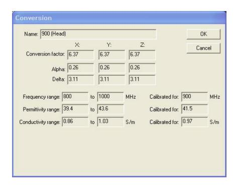
The target permittivity and conductivity at 835 MHz is 41.5 and 0.90 respectively which is within the calibrated range of the probe parameter. The following parameters are declared in the probe calibration certificate on page 8:
