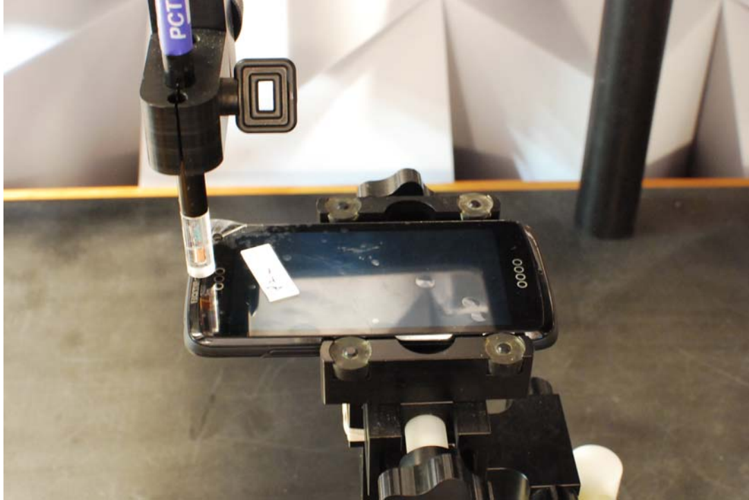
Figure 13-1 Test Setup for Wireless Device
