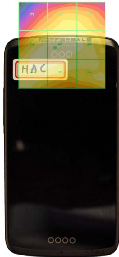
Figure 17-5 H-Field WD Scan overlay
