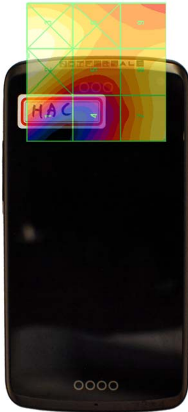
Figure 17-4 E-Field WD Scan overlay
