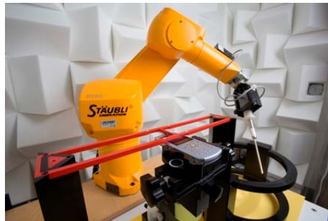
Figure 5-5 SPEAG Robotic System
