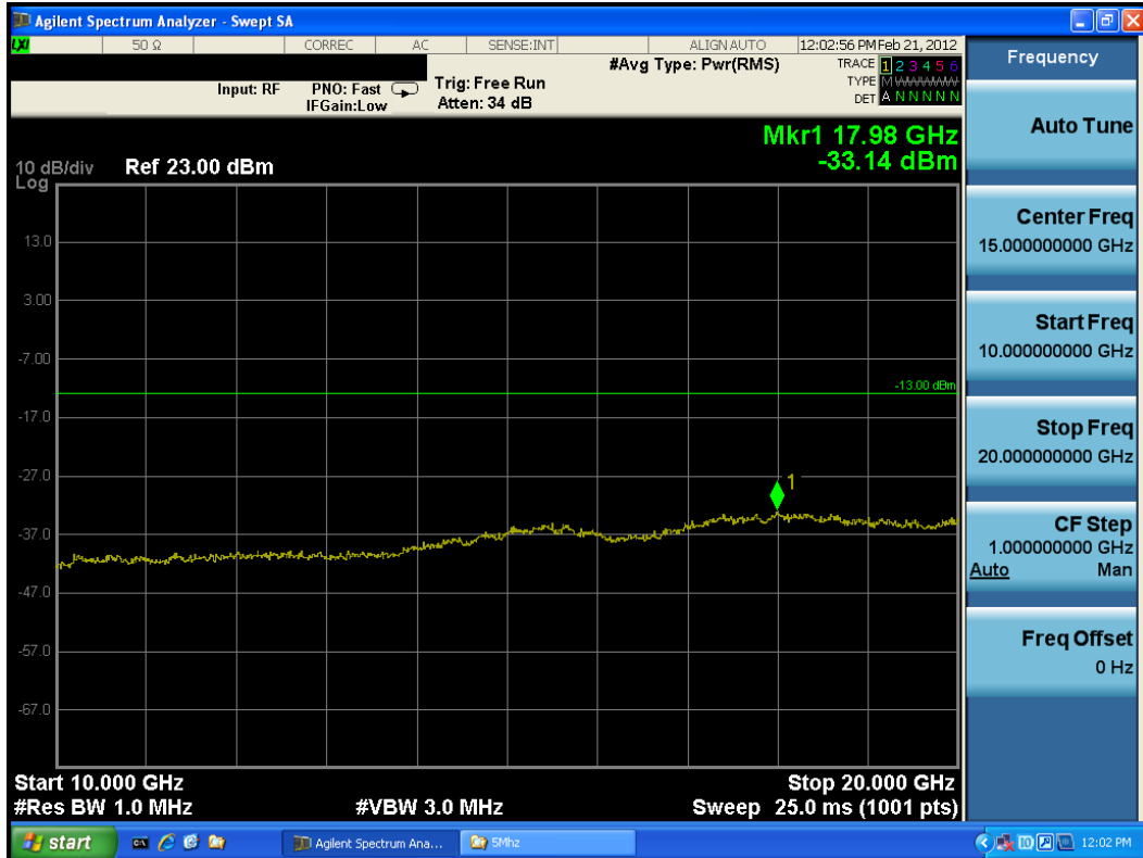
Plot 9-14. Conducted Spurious Plot (5MHz QPSK – RB Size 1, RB Offset 0 – High Channel)
