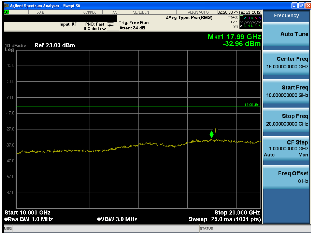
Plot 10-10. Conducted Spurious Plot (5MHz QPSK – RB Size 1, RB Offset 0 – Low Channel)
