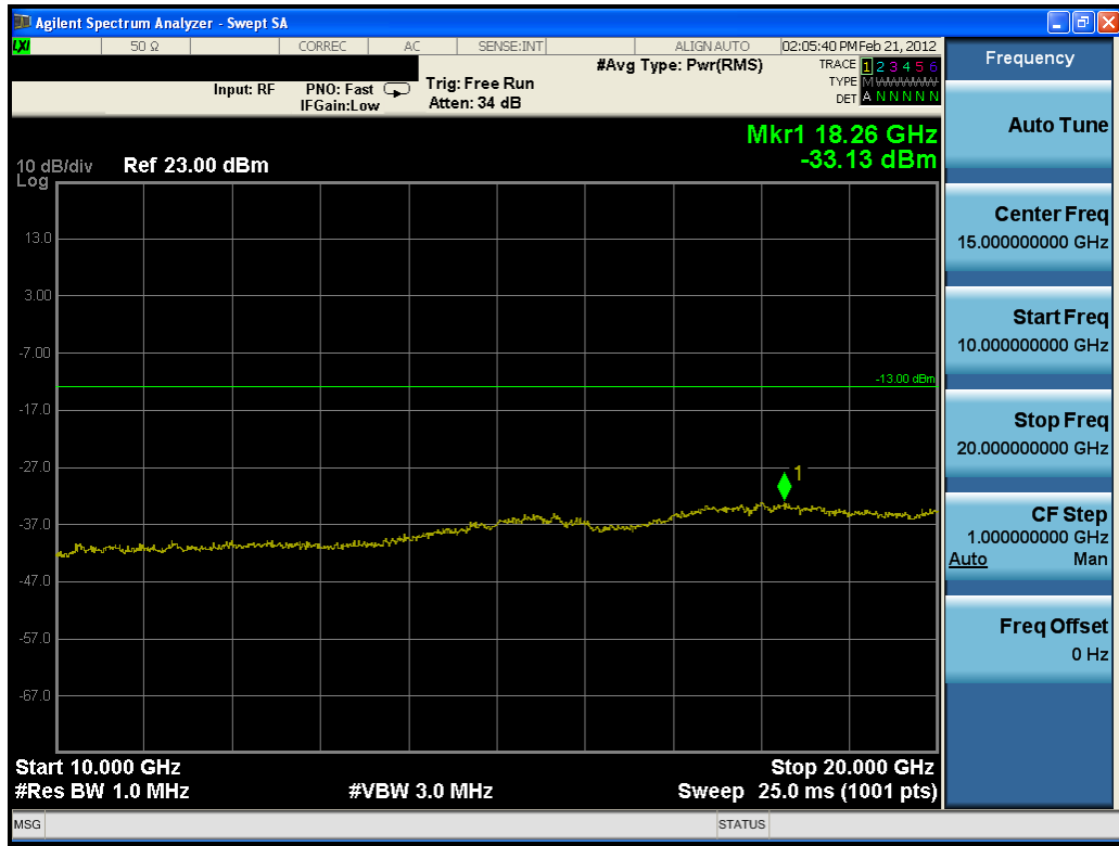
Plot 10-20. Conducted Spurious Plot (10MHz QPSK – RB Size 1, RB Offset 0 – High Channel)
