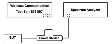
(Configuration of conducted Emission measurement) Test Procedure
