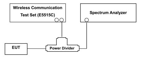
(Configuration of conducted Emission measurement) Test Procedure
