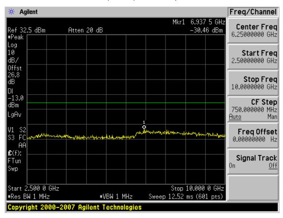
■ GSM1900 MODE (512 CH.) Conducted Spurious Emissions1
