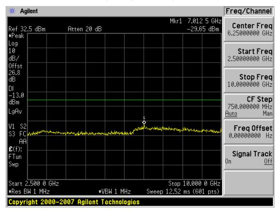
■ GSM850 MODE (251 CH.) Conducted Spurious Emissions1
