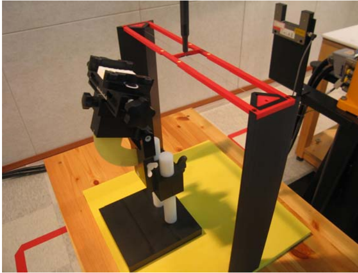
Figure 2. HAC Phantom & Device Holder
