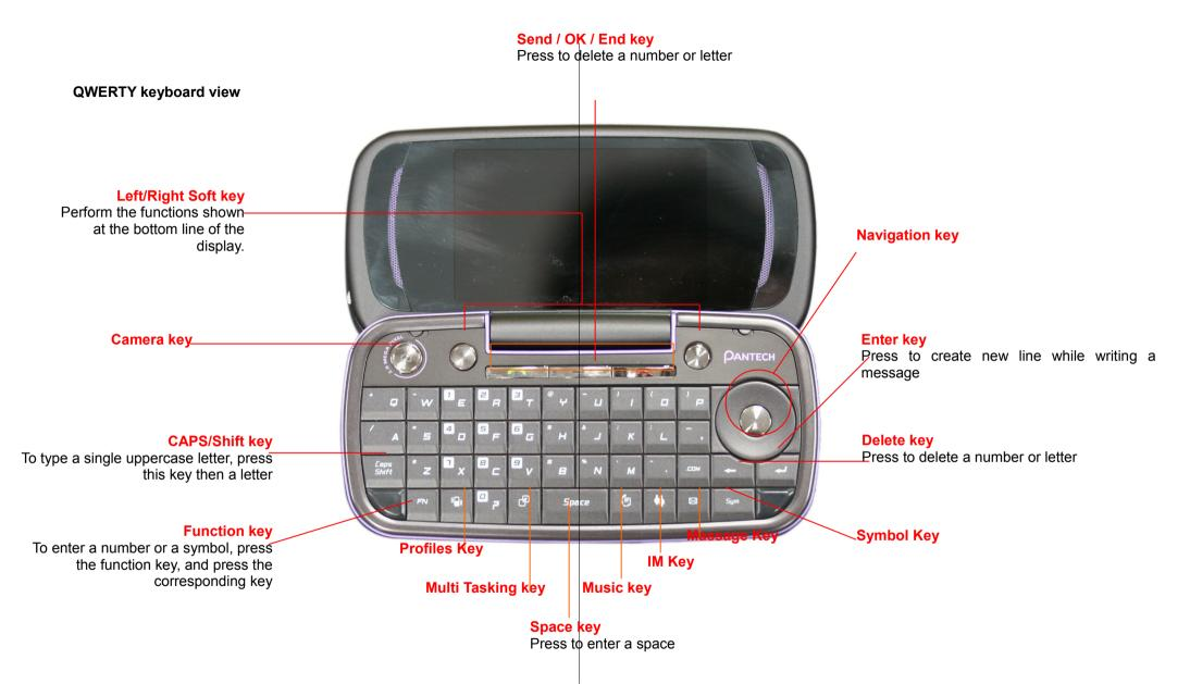
Note: To use the QWERTY keyboard, ensure that the Number pad is closed, then hold the phone horizontally and slide the screen up.
