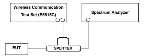
(Configuration of conducted Emission measurement)
