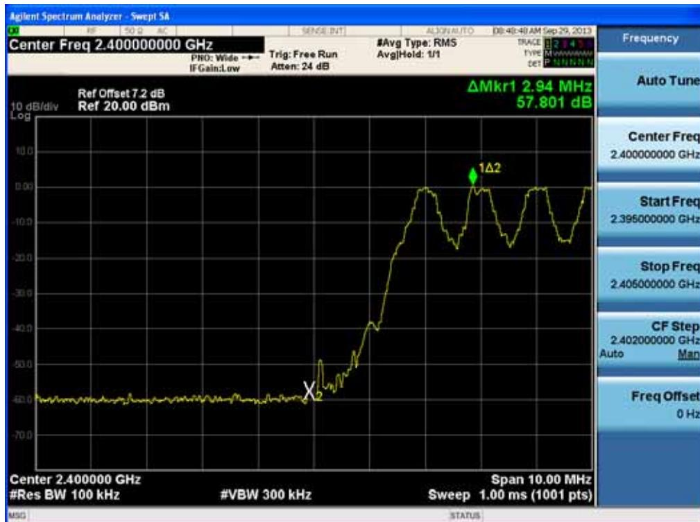
Test Plots with hopping (GFSK)
