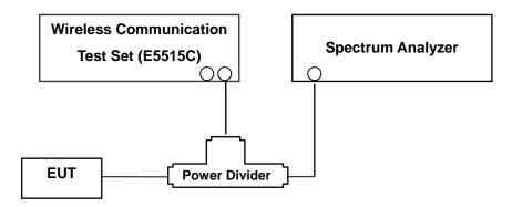
(Configuration of conducted Emission measurement) Test Procedure
