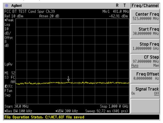
Test Plots (8DPSK) - 30 MHz - 1 GHz (RBW:100 kHz, VBW: 300 kHz) Spurious Emission (High-CH)
