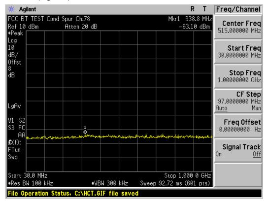
Test Plots (8DPSK) - 30 MHz - 1 GHz (RBW:100 kHz, VBW: 300 kHz) Spurious Emission (Low-CH)
