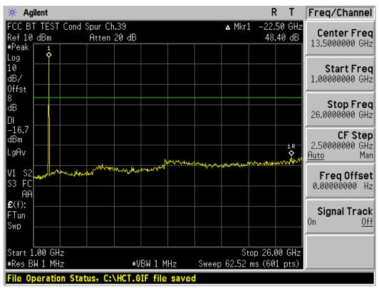
Test Plots (8DPSK) - 1 GHz - 26 GHz (RBW:1 MHz, VBW: 1 MHz) Spurious Emission (High-CH)
