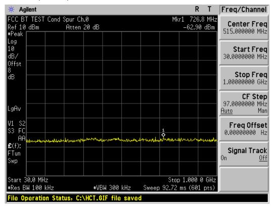
Test Plots (GFSK) - 30 MHz - 1 GHz (RBW:100 kHz, VBW: 300 kHz) Spurious Emission (Mid-CH)
