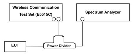
(Configuration of conducted Emission measurement) Test Procedure
