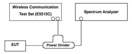
(Configuration of conducted Emission measurement) Test Procedure
