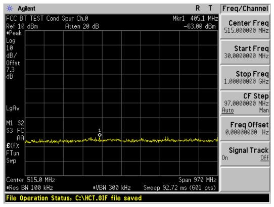
Test Plots (GFSK) - 30 MHz - 1 GHz (RBW:100 kHz, VBW: 300 kHz) Spurious Emission (Mid-CH)
