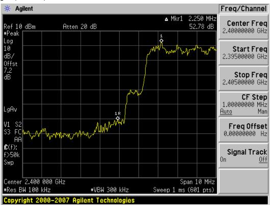
Test Plots with hopping (8DPSK) Band Edges (High-CH)
