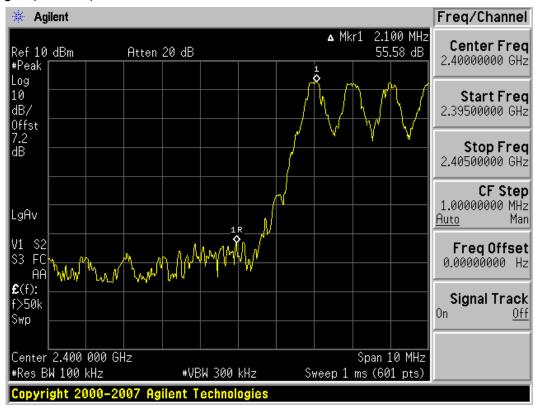
Test Plots with hopping (GFSK) Band Edges (High-CH)
