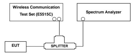
(Configuration of conducted Emission measurement)
