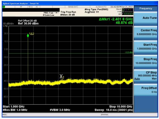
Test Plots (GFSK) - 1 GHz - 10 GHz Spurious Emission (Mid-CH)
