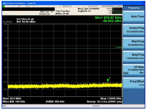
Test Plots ( $\pi$ /4DQPSK) - 30 MHz - 1 GHz Spurious Emission (Mid-CH)
