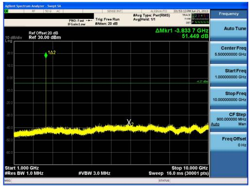
Test Plots (8DPSK) - 1 GHz - 10 GHz Spurious Emission (Low-CH)
