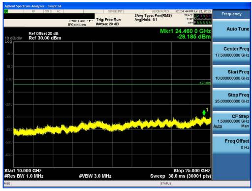
Test Plots (8DPSK) - 10 GHz - 25 GHz Spurious Emission (Low-CH)
