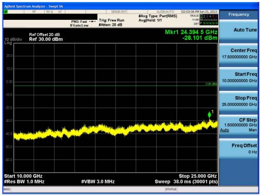
Test Plots (8DPSK) - 10 GHz - 25 GHz Spurious Emission (High-CH)
