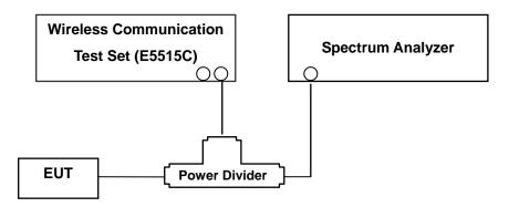
(Configuration of conducted Emission measurement) Test Procedure
