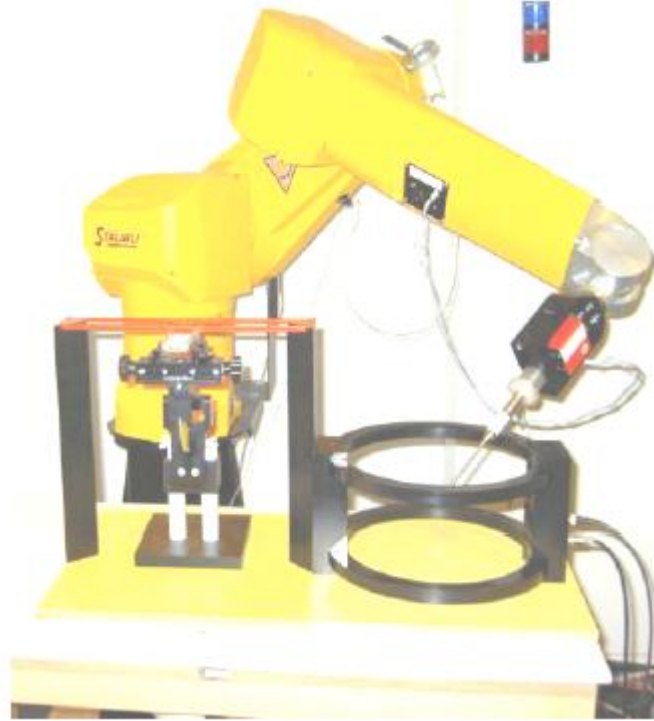
Figure 1: T-Coil setup with HAC Test Arch and AMCC.
