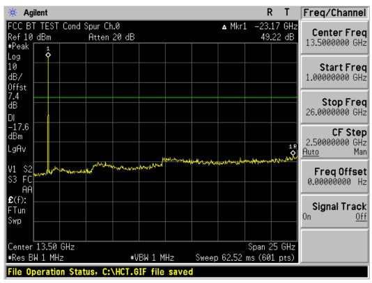
Test Plots (GFSK) - 1 GHz - 26 GHz (RBW:1 MHz, VBW: 1 MHz) Spurious Emission (Mid-CH)
