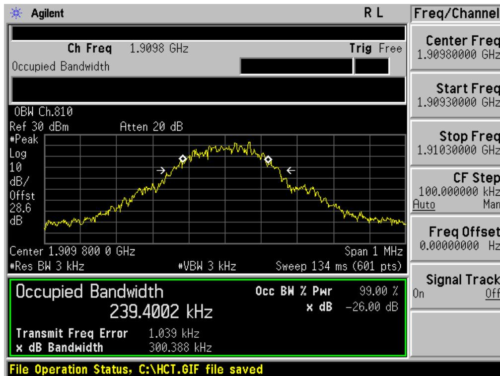
■ GSM1900 EDGE (661 CH.) Occupied Bandwidth
