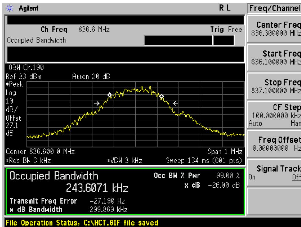
■ GSM850 MODE (251 CH.) Occupied Bandwidth
