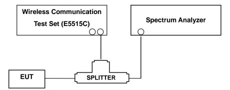
(Configuration of conducted Emission measurement)
