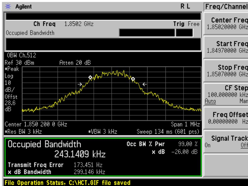
■ GSM1900 MODE (661 CH.) Occupied Bandwidth
