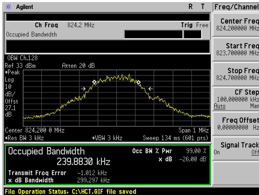
■ GSM850 MODE (190 CH.) Occupied Bandwidth
