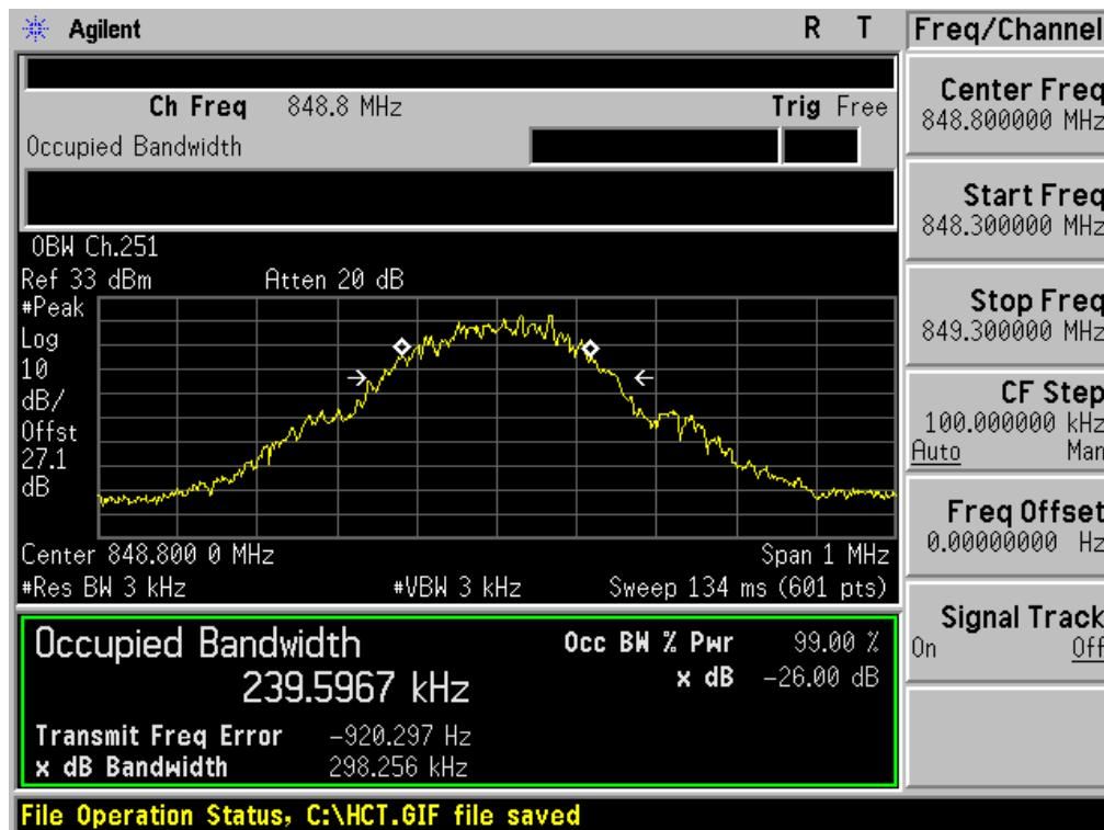
■ GSM850 EDGE (190 CH.) Occupied Bandwidth
