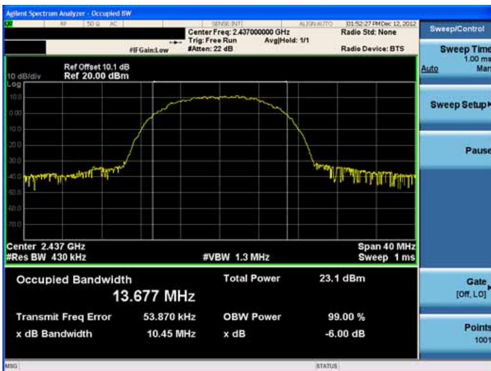
6dB Bandwidth plot (802.11b-CH 6)
