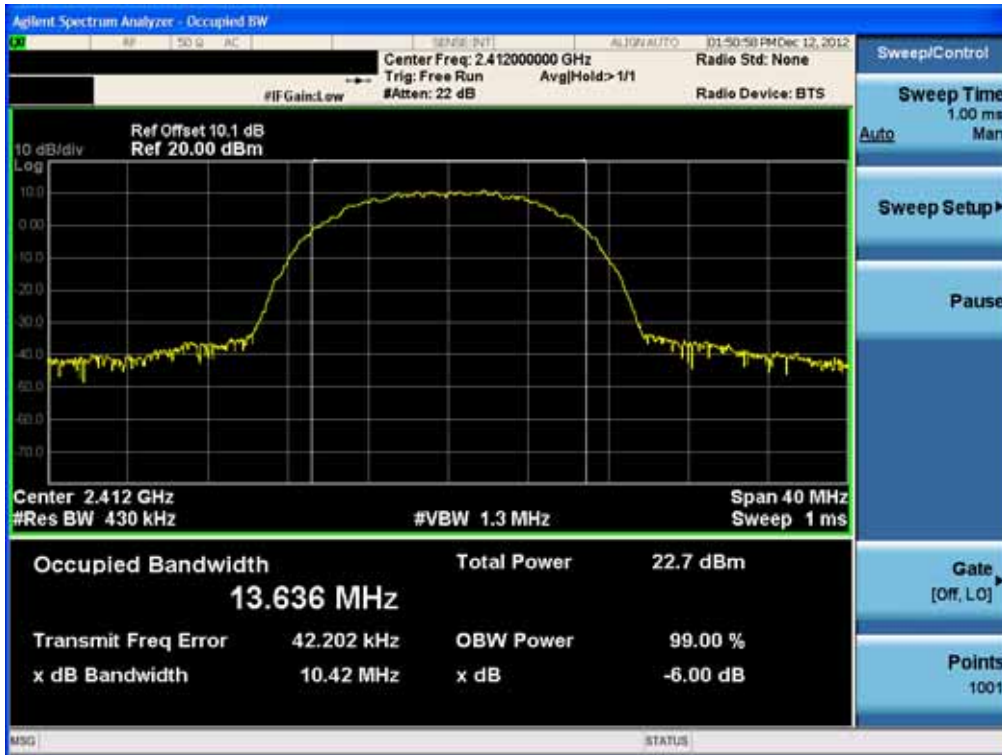
6dB Bandwidth plot (802.11b-CH 6)
