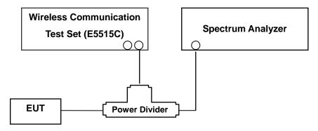
(Configuration of conducted Emission measurement) Test Procedure
