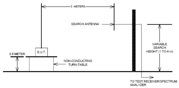
The measurement facilities used for this test have been documented in previous filings with the commission pursuant to section § 2.948. The Fully-anechoic chamber meets requirements in ANSI C63.4 –2003. A mast capable of lifting the receiving antenna from a height of one to four meters is used together with a rotatable platform mounted at three from the antenna mast.
