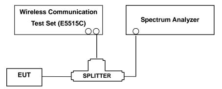
(Configuration of conducted Emission measurement)
