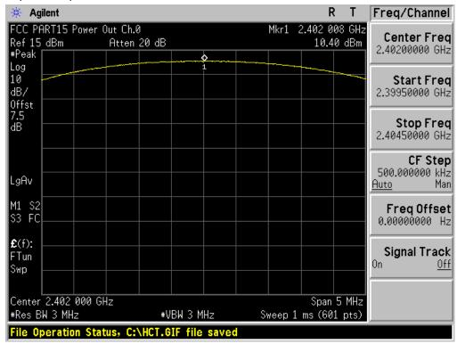
Test Plots (π/4DQPSK) Peak Power (Mid-CH)
