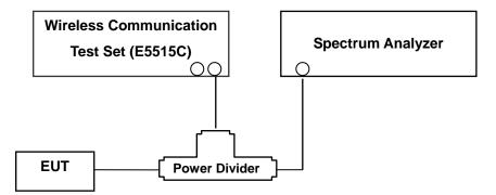
(Configuration of conducted Emission measurement) Test Procedure
