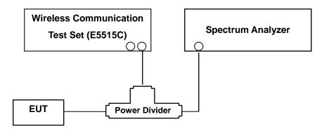
(Configuration of conducted Emission measurement) Test Procedure
