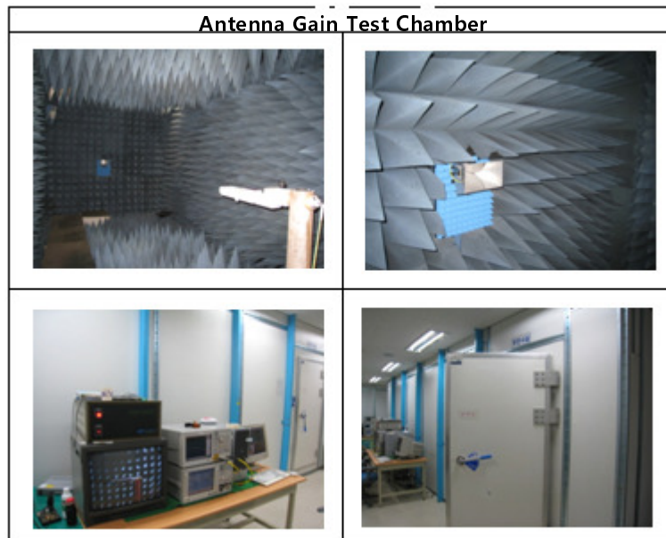
[ Picture 2- 8] Antenna Gain Test
