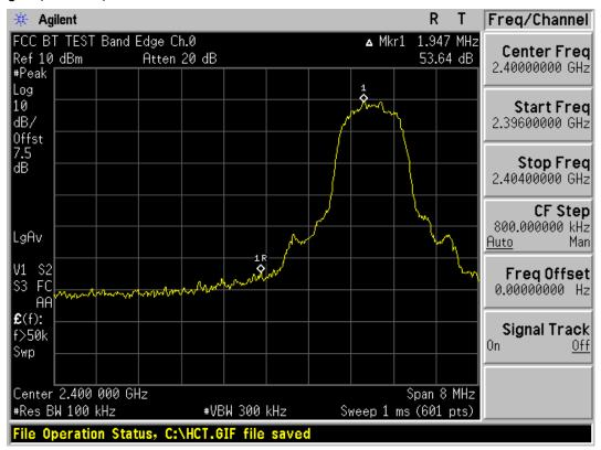
Test Plots (8DPSK) Band Edges (High-CH)
