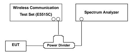
(Configuration of conducted Emission measurement)
