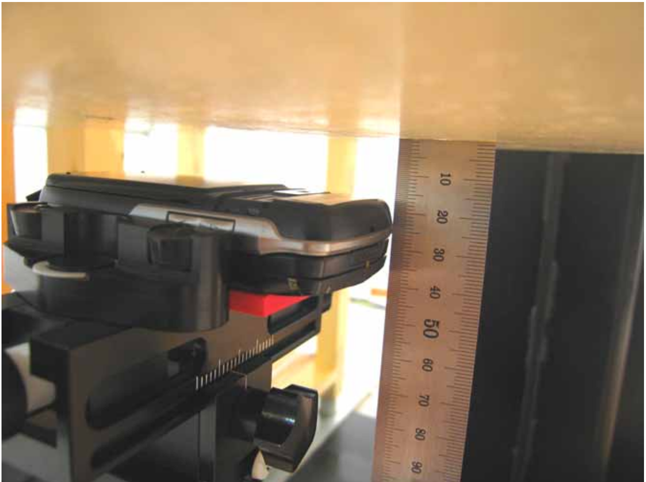
[Distance of 1.5 cm from the EUT] Headset was connected with the bottom port of the EUT.
