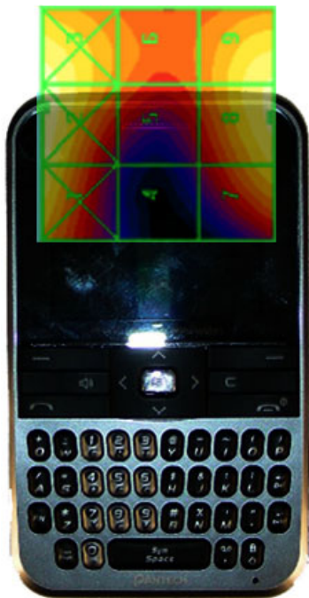
Figure 16-4 E-Field WD Scan overlay
