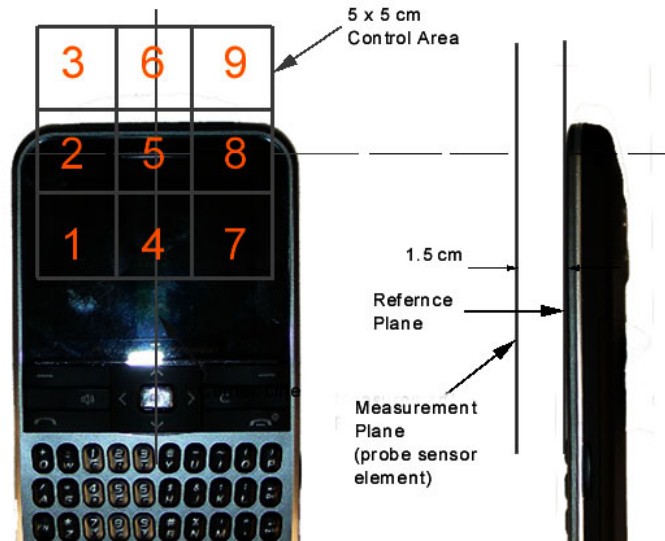
Figure 16-3 5x5 Scan grid above WD
