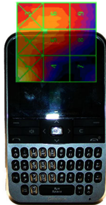
Figure 16-5 H-Field WD Scan overlay
