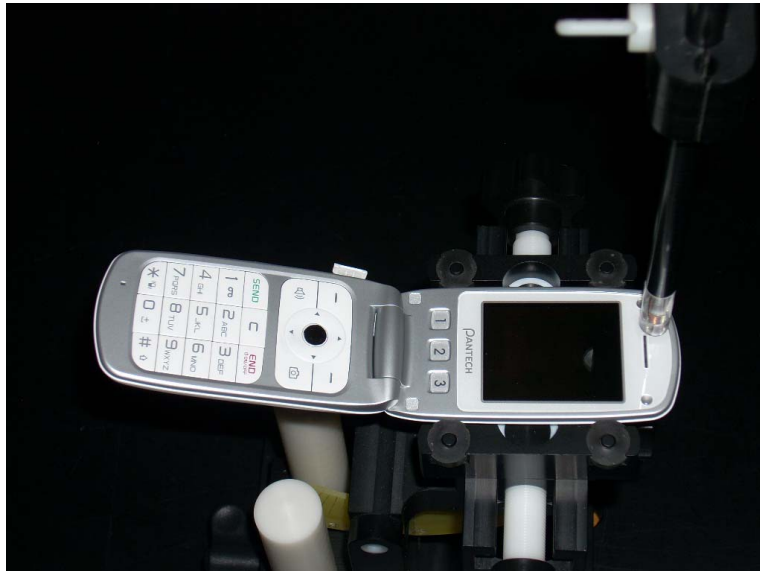
Figure 12-2 Test Setup for Wireless Device
